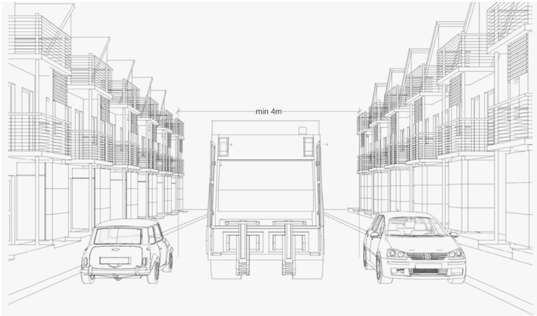
Diagram 6.3 – An example of minimum road width clearance required where on-street parking is provided for on both sides of the road
