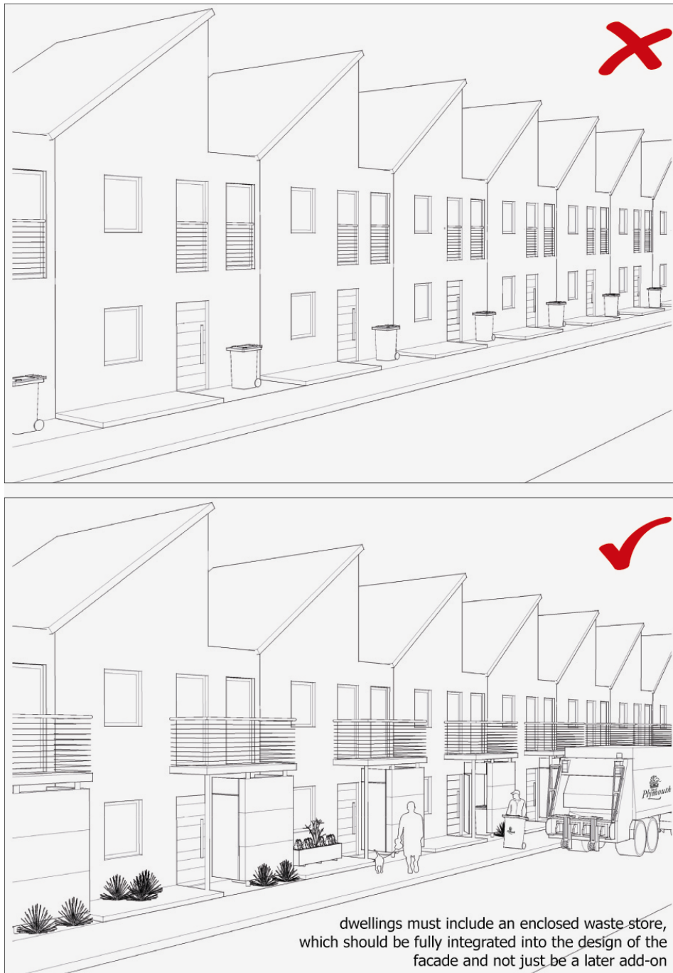
Diagram 6.2 – Good and poor examples of provision for bin storage in residential design
